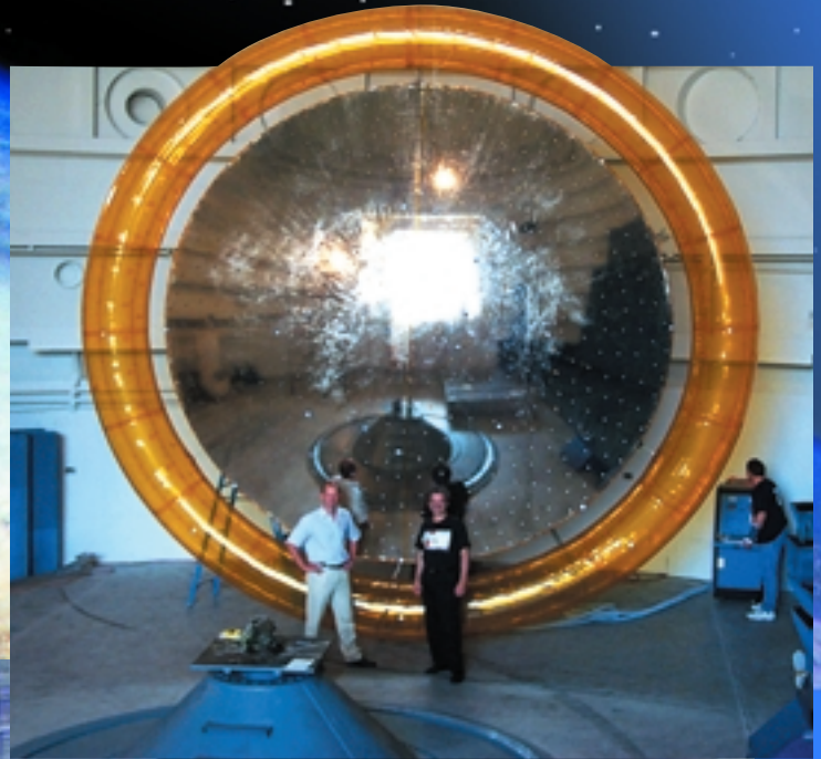
ABOVE 5-m-diameter inflatable parabolic reflector in NASA Langley Research Center's 16-m vacuum chamber.
